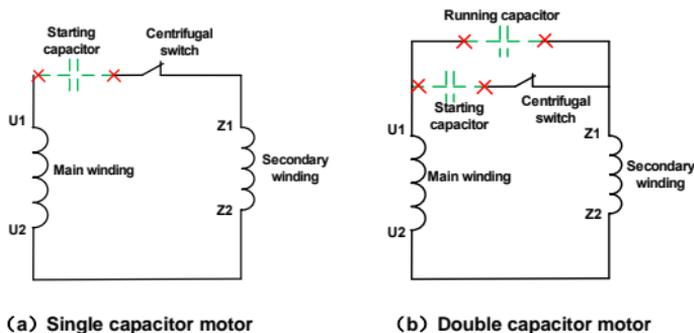
Internal wiring of the single-phase motor winding after removing the starting and running capacitor:
