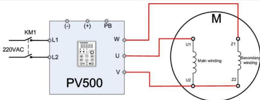
U2 and Z2 are the common terminals of the windings. Connect them to the output terminal V of the solar pumping inverter. Connect U1 to the output terminal U of the inverter. Connect Z1 to the output terminal W of the inverter. (**Note:** Use the screws equipped with the inverter.) Connect DI4 of the inverter to COM in short circuited manner.
