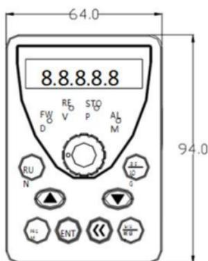
Figure 4-1 Keypad diagram for inverters
